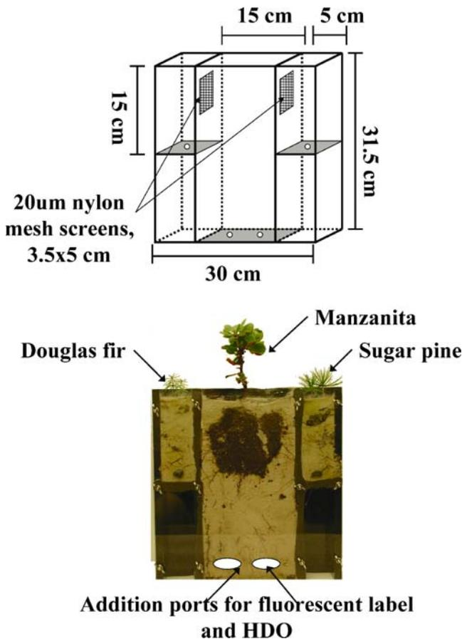
**Fig. 1** Diagram (a) and photograph (b) of one of the mesocosms. The sizes of the different compartments and location of the root barriers are shown in a. Positions of the ports where the dye and isotope labels were injected are shown in b
