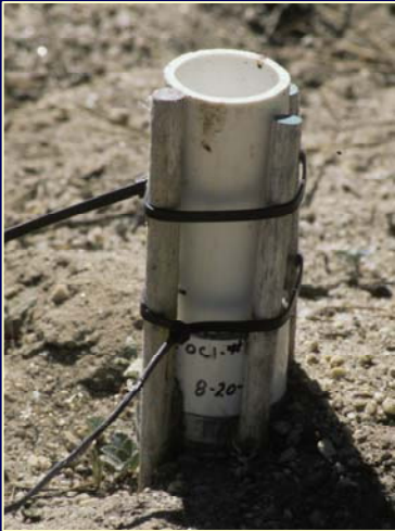
Through-fall sampler for measuring atmospheric inputs
