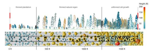
*Measurements:* The high-frequency laser pulses can penetrate the upper canopy providing a much fuller measure of a forest's three-dimensional structure. LiDAR is less accurate at measuring sub-canopy conditions such as ladder and ground fuels unless the forest is open or a high-density of laser pulses are acquired (see considerations). LiDAR, however, can be combined with ground-based measurements of the forest floor to improve fuels assessments.
