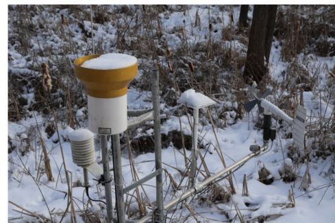
Fig. 2. Snow blanketed the rain gauge and pyranometer on January 22, 2024, at a microclimatic station in East Lansing, Michigan, during a week-long snowfall period.
